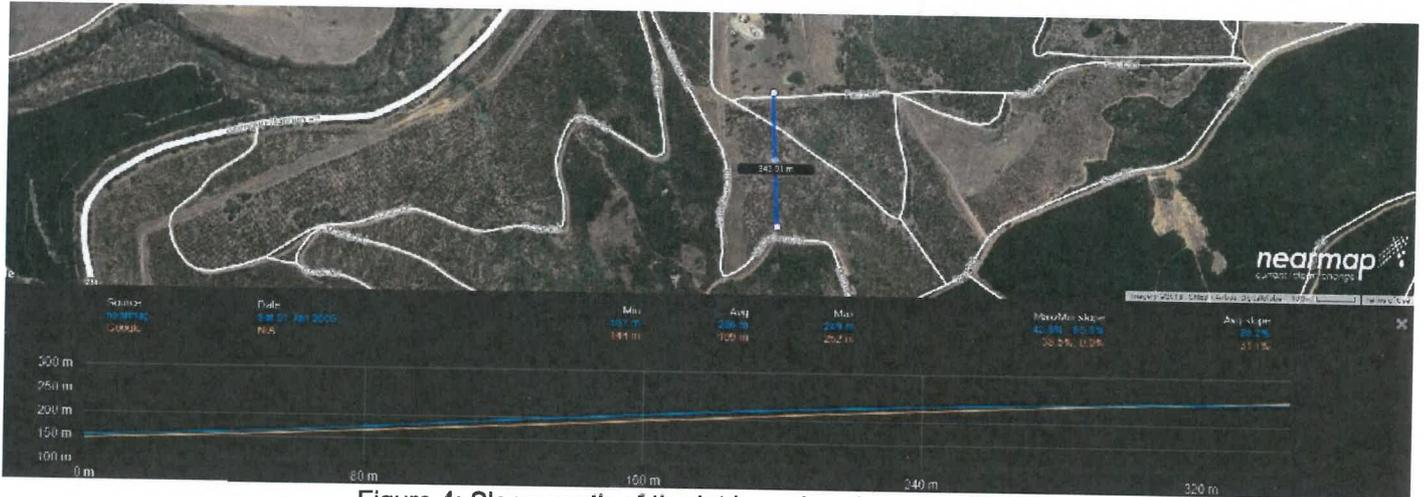
Figure 4: Slope south of the lot boundary (upslope 17.28°).
